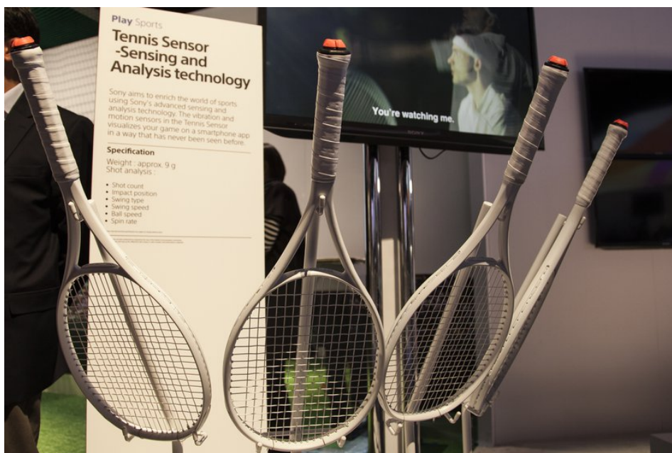
Sony developed a sensor for tennis that measures swing speed, spin and other
